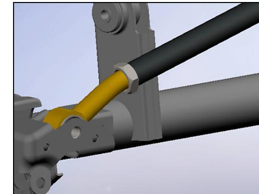
**HINT:** Bend in axle (gold) end of trackbar must point up to prevent interference from occurring when suspension articulates.
