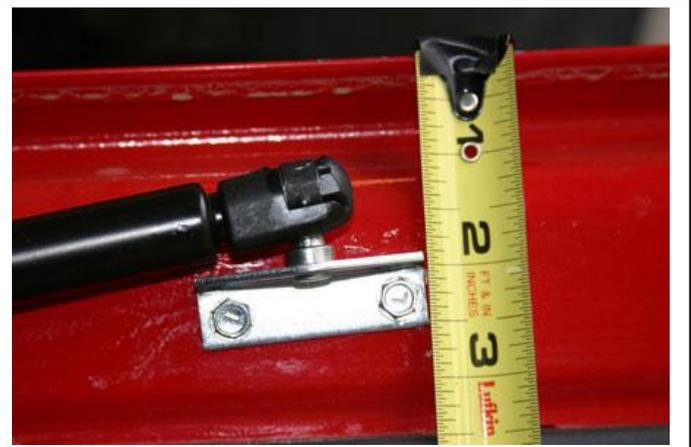
Go ahead and drive in both screws, using the supplied star washers.
