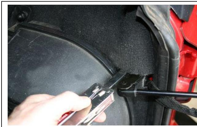
2. If you have the large speaker in the rear, remove the (3) 15mm nuts holding it on and set it aside. You don't have to disconnect it, just get it out of the way.
