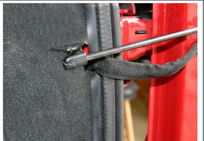
6. With the tailgate pushed (by you) against the Jeep's stop, mark the location of the outer (small) bracket. The outermost screw should be 2 ¼ inches from the top of the tail gate. The other screw should be about 3/8" lower. The one you see here is only ¼" lower. You will be able to easily see where it goes by putting in the outer screw first, then aligning the bracket with the slanted spring.
