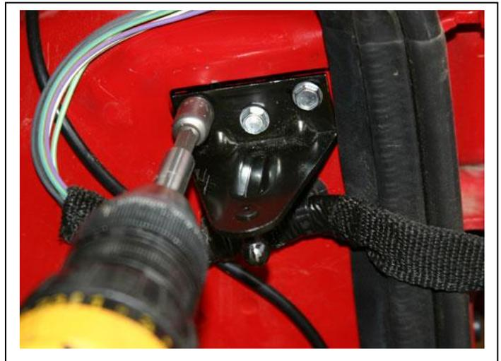
5. Snap on the small end of the gas spring. Open the tailgate all the way to the stop so you can position the small bracket. You will be installing that bracket so the spring pushes the tailgate all the way to the Jeep's stop.
