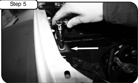
Loosen 10mm bolt holding in airbox bracket. Save for later install.
