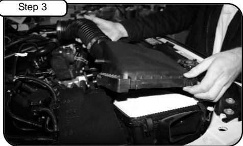
Disconnect crank case line at OE airbox. Disconnect OE clips holding in upper half of OE airbox. Remove upper half of airbox from vehicle.
