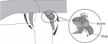
Threading Strap through Buckle
