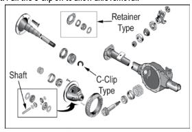
This is a good time to inspect your differential for metal shavings, wear, etc. Inspect your bearings and seals. If necessary, the following components are available from your CROWN Dealer:
