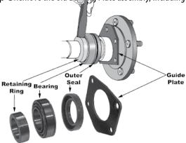
Wheel Cylinders, etc. Clean and inspect the Bearing surfaces.
