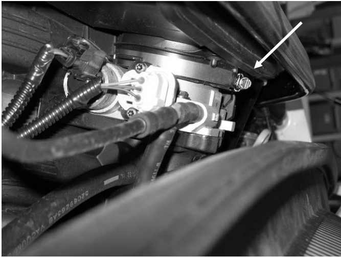
i) Loosen the throttle body hose clamp.
