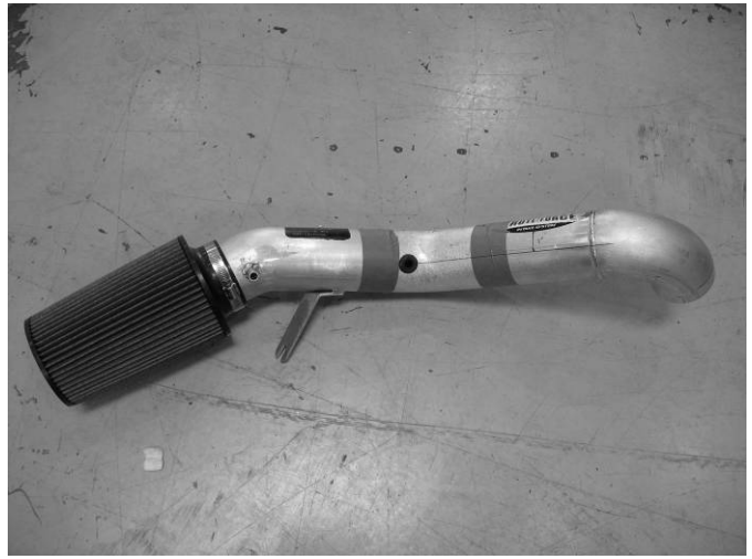
i) Attach the filter element as shown. Secure with #60 hose clamp.
