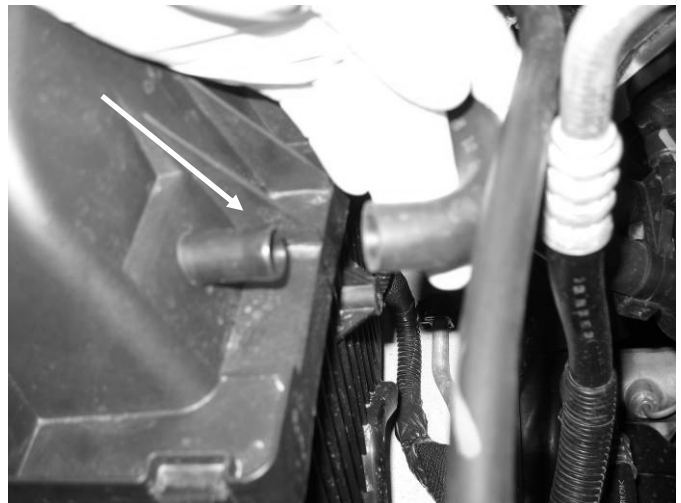
d) Disconnect the crankcase breather hose.
