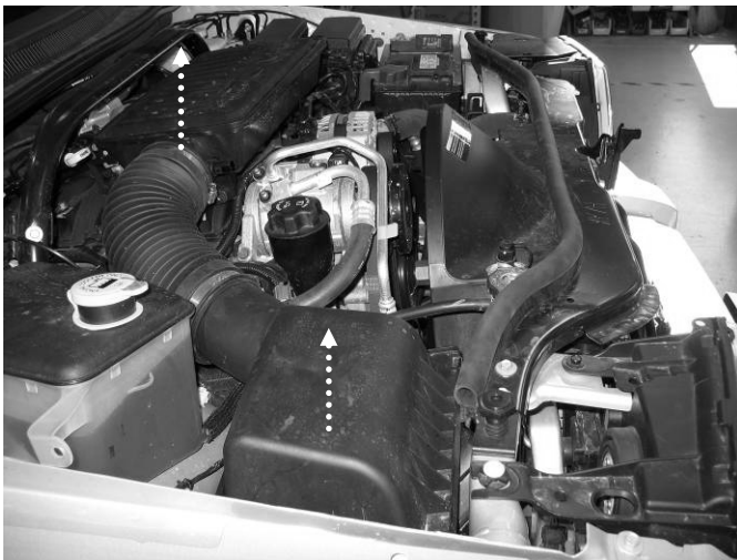
o) Remove the air box assembly.
