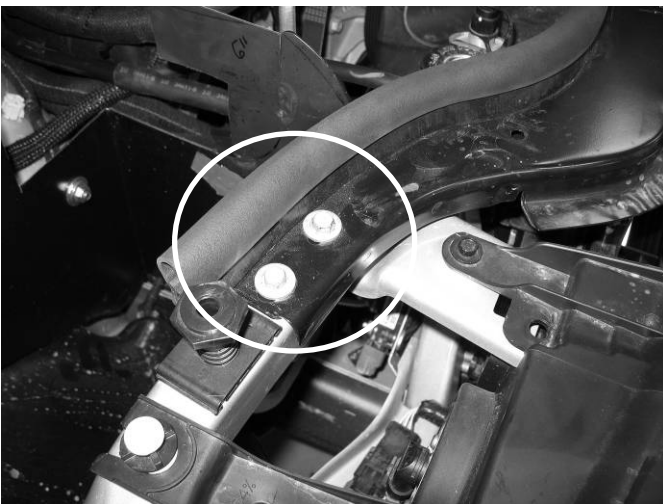
f) Insert the heat shield tab underneath the hood latch support bracket. Secure with factory hardware.
