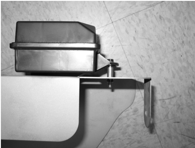
p) If your truck comes equipped with cruise control, reinstall the vacuum canister as shown. Use the M6 bolt, washer, nipple and M6 nut provided.
