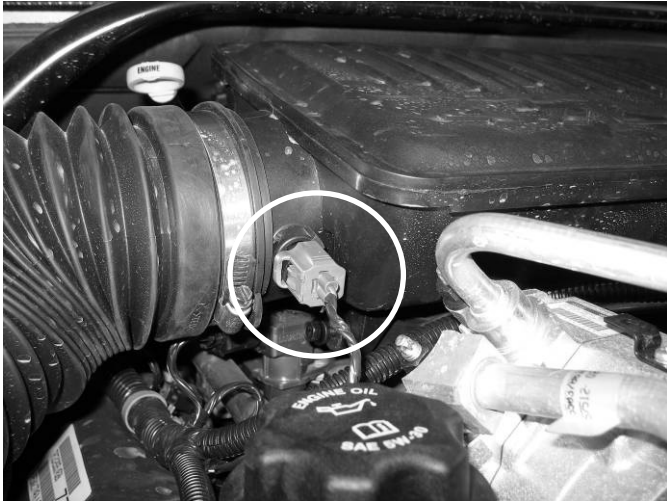
a) Disconnect the Inlet Air Temperature sensor.
