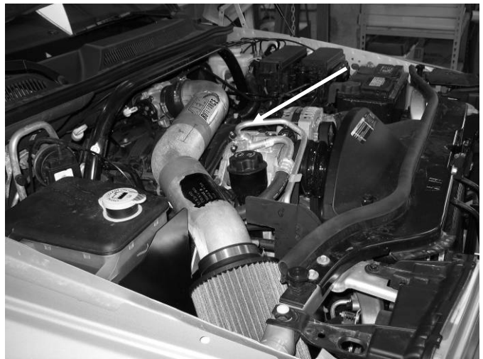
k) Insert the inlet pipe as shown.
