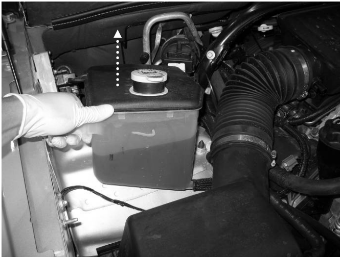
g) Gently remove the coolant reservoir from its factory location and set aside. Do not disconnect coolant lines.
