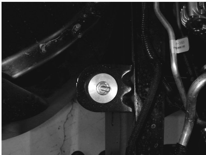
a) Assemble the heat shield mount to the air box mounting tab. Refer to the following diagram, using the 1/4-20 bolt, washer, spacer, and nut. Reuse the rubber grommet from the air box mounting tab.
