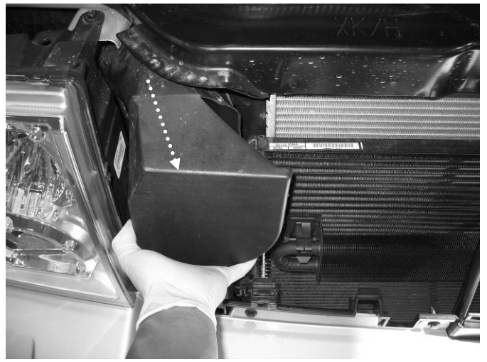
n) Disconnect the resonator inlet. Pull straight forward.
