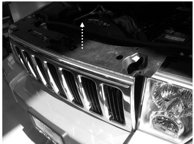
l) Remove the grill. Lift the grill up and pull forward.
