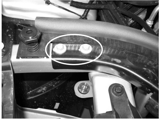
c) Loosen and remove the bolts to the hood latch support bracket. These will be reused.
