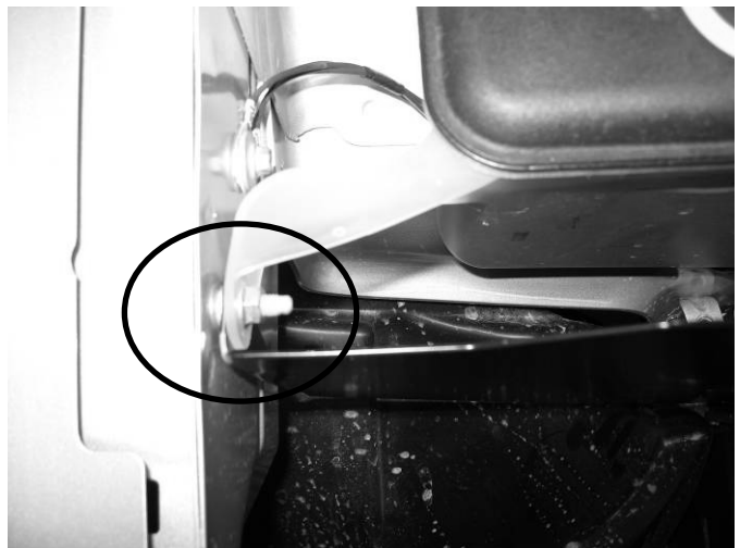
g) Secure the heat shield tab between the fender and the coolant overflow reservoir with M6 washer and nut. Secure reservoir.
