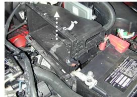
**h)** Pull up on the other half of the air box. Remove the air box.
