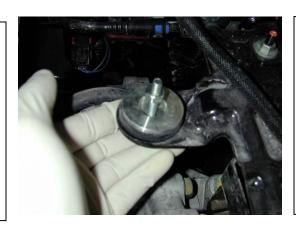
e) Insert the spacer over the bolt. Secure the thread bolt with the provided nut. Center the spacer in the grommet and tighten.
