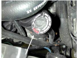
**d)** Loosen hose clamp of the inlet tube at the throttle body.
