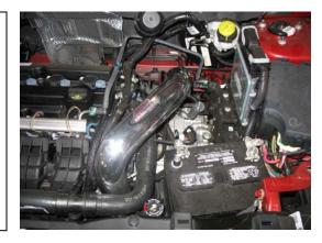
**g)** Insert pipe as shown. Line up the bracket to the spacer assembly.
