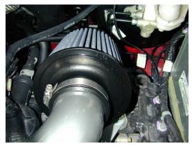
i) Attach filter. Check for clearance and tighten with filter hose clamp.
