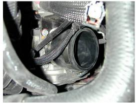
**b)** Attach the reducer coupler to the throttle body. Secure with the 2.5" hose clamp. Loosely attach the 2.75" hose clamp to the other side of the coupler.
