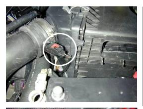
e) Remove IAT (Intake Air Temperature) Sensor harness connector. Pull tab out, then depress clip.
