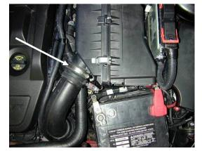
**c)** Loosen hose clamp at the air box.
