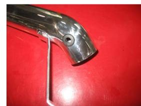
**c)** Insert grommet for the IAT sensor into the inlet pipe.
