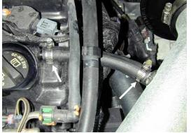
I) Attach the breather hose as shown to the inlet pipe and to the crankcase vent. Secure with hose clamps.
