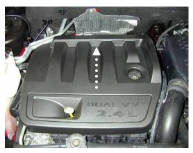
**a)** Remove engine cover by pulling straight up.
