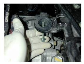
**d)** Insert the all thread bolt with ¼" washer up through the air box mount grommet.
