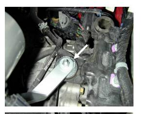
**j)** Check for clearance of the inlet pipe around the coolant hose. Tighten bracket with washer and lock nut.
