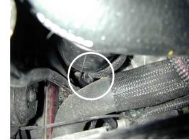
**f)** Remove Christmas Tree Mount zip tie from inlet tubing. Remove inlet pipe. Remove IAT Sensor.
