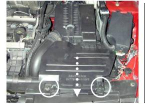
**b)** Twist and remove retaining clips. Remove ducting by pulling up and forward.
