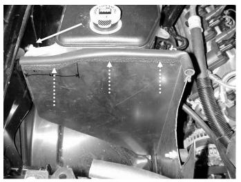
c) Insert heat shield as shown. Line up mounting hole at the coolant reservoir and tighten with M6 Nylok nut. Attach rubber foam gasket.
