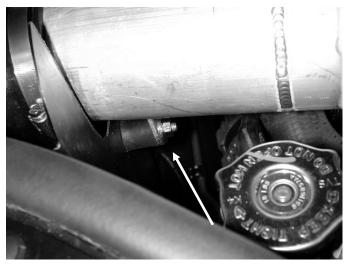
i) Check pipe clearance at the heat shield. Check clearance around the filter. Secure the inlet pipe with the supplied washer and M8 Nylok nut.
