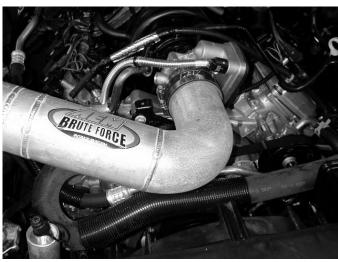
j) Insert inlet pipe as shown into the coupler at the throttle body.
