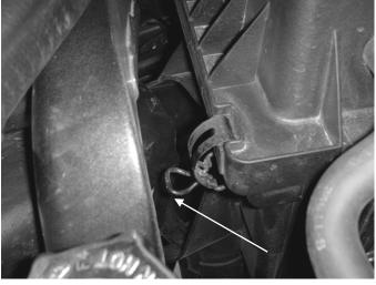
**I)** Disconnect the air tube on the lower half of the air box by pulling towards the front of the vehicle.
