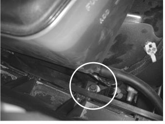
**h)** There is a bolt located between the coolant reservoir and the air box. Loosen and remove this bolt in order to remove the air box.
