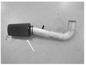
i) Attach the filter element and secure.
