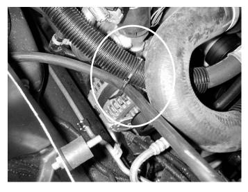
**g)** Zip tie the A/C line to the coolant overflow return line. Make sure not to pinch the hose.
