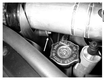
k) Rotate the inlet pipe counter clockwise. Align mounting bracket to the installed rubber mount.
