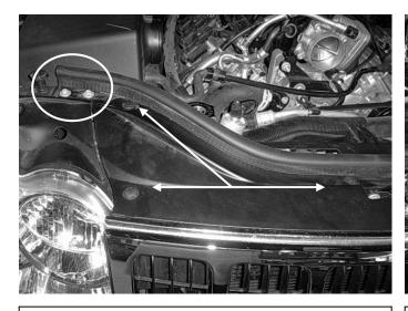
**i)** Remove tabs from the front the grill. Loosen and remove the grill mounting bolts.
