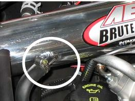
I) Rotate breather hose 90 degrees clockwise. Reattach the crankcase breather hose. Secure with provided hose clamp.
