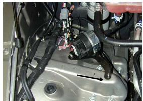
g) Loosen and remove mounting nut. This nut will be reused if your vehicle has cruise control. If your vehicle is not equipped with cruise control, then use the M6 nut provided.
