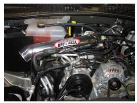
j) Insert the inlet pipe as shown. Align with mounting bracket.
