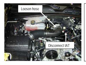
a) Loosen the hose clamp at the throttle body. Disconnect the IAT (Inlet Air Temperature) Sensor harness connector. Push out the clip on the IAT to release.
