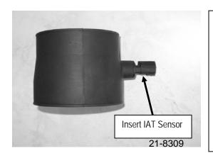
b) Remove the IAT Sensor from the stock inlet pipe. Reinsert the sensor into the new throttle body coupler as shown.
