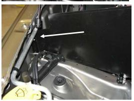
h) Insert the heat shield. Secure with provided washers and nuts. Check for factory installed hardware. If studs are secured with nuts already, remove first. Careful not to damage vacuum hoses or wire harness
