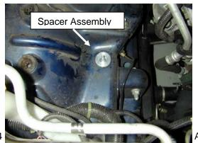
c) Mount the spacer assembly in the lower rubber mount left by the bottom of the air box. Spacer assembly consists of the bolt, washer, spacers and nut. Refer to diagram.
