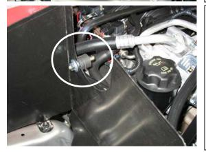
i) Attach the rubber mount and secure with 8mm washer and nut.
