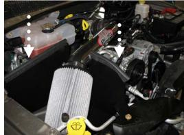
m) Attach filter and secure. Attach rubber foam gasket to the top of the heat shield.
