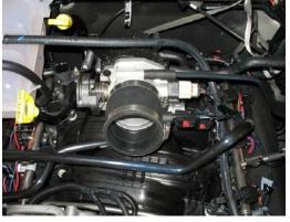
f) Attach coupler as shown. Secure with #52 hose clamp on the throttle body and #48 on the open end. Reattach the IAT Sensor harness.
