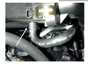
b) Disconnect the crankcase breather hose from the air box. Remove air box by pulling straight up.
