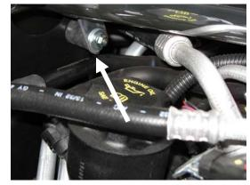
k) Secure bracket with 8mm washer and nut.
