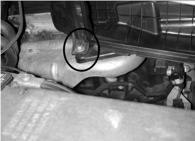
e) Remove the nut securing the air filter housing to the engine.
