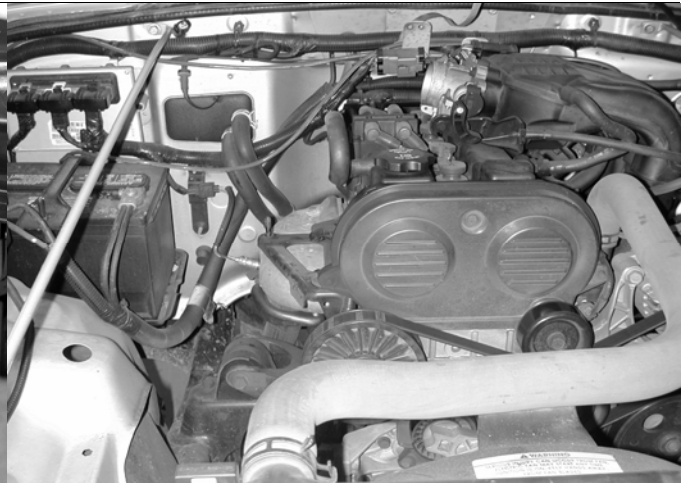
f) Remove the air filter housing from the engine compartment.
