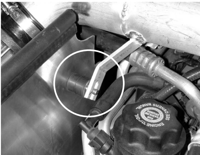
i) Secure bracket to the rubber mount on the heat shield with provided washer and lock nut. Refer to diagram on next page.
