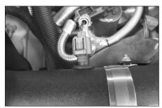
18. Install the short edge trim onto the heat shield assembly as shown. NOTE: Some trimming of the edge trim may be necessary.
