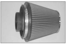
33. Install the filter adapter into the air filter as shown, secure with the provided hose clamp.
