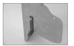
16. Install the large "L" bracket (26626) onto the heat shield as shown with the provided hard-ware.
