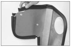
19. Install the long edge trim onto the heat shield assembly as shown. NOTE: Some trimming of the edge trim may be necessary. 25. Install the tube mounting bracket assembly onto the plenum mount and secure with the factory nut removed in step #23.
