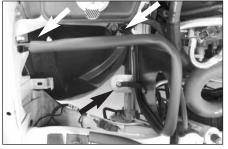
21. Install the heat shield assembly into the vehicle and secure to the lower and upper air box mounts and washer bottle stud with the provided hardware.
