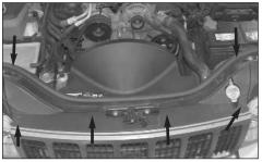
10. Using a small screwdriver, release the center holding pins in the six grill retaining clips shown.
