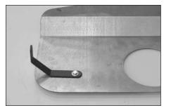
15. Install the supplied "C" bracket (07171) onto the heat shield as shown with the provided hardware.
