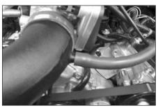
31. Install the provided crank case vent hose onto the valve cover and then onto the K&N intake tube as shown.
