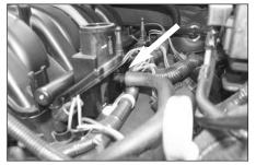
8. Remove the crank case vent hose from the engine as shown.
