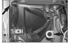
20. Remove the coolant reservoir-retaining nut and air box mounting grommet shown.
