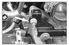
23. Remove the nut, which secures the intake plenum-mount shown. **NOTE: This nut will be reused.**
