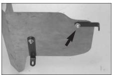
17. Install the small "L" bracket (07158) onto the heat shield as shown with the provided hardware.
