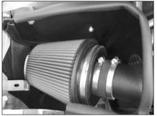
35. Install the K&N air filter assembly onto the K&N intake tube as shown and secure with the provided hose clamp.
