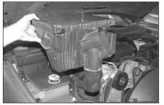
14. Lift the lower air box and remove it from the vehicle as shown.
