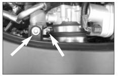
4. Remove the intake plenum-mounting bolt and loosen the intake plenum hose clamp at the throttle body.
