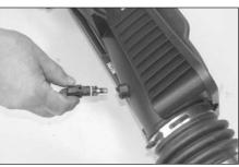
27. Rotate the air temperature sensor counter clockwise and remove the sensor from the stock intake plenum as shown. NOTE: Be very careful with the air temperature sensor, as it is very fragile.
