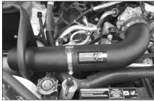
30. Install the K&N intake tube into the silicone hose at the throttle body and onto the saddle clamp, then secure with the provided hose clamps.
