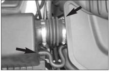
2. Loosen the hose clamp, which secures the stock intake tube to the intake plenum, and disconnect the crank case vent hose form the air box lid.
