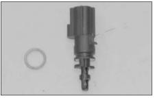
28. Remove the rubber sealing "O" ring from the air temperature sensor as shown.
