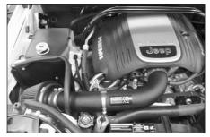
37. Reinstall the engine cover, reconnect the vehicle's negative battery cable. Double check to make sure everything is tight and properly positioned before starting the vehicle.
