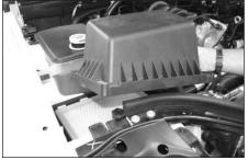
9. Un hook the air box lid retaining clamps and then remove air box lid and filter. **NOTE: K&N recommends that you do not discard your factory air intake.**
