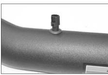
29. Install the air temperature sensor into the K&N intake tube as shown. NOTE: Be careful with the air temperature sensor, as it is very fragile.
