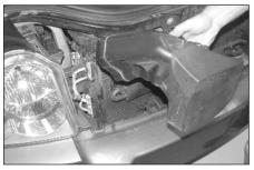
12. Pull the fresh air duct forward to disconnect it from the air box and then remove it from the vehicle.
