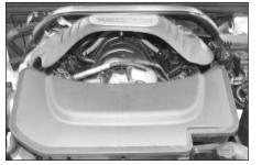
3. Remove the oil filler cap and then lift up the front of engine cover to gain access to the
