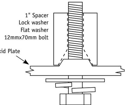
1. 2003-current TJ Wranglers- Install the six spacers (1.25"OD x 1.25" tall) between the frame and the cross member with the flat end of the spacer up against the frame. The 1/2" lock washer goes onto the M12 x 1.75 x 70 bolt first followed by the 1/2" flat washer.
