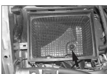
8. Remove the air box mounting bolt
