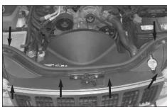
5. Using a small screwdriver, release the center holding pins in the six grill retaining clips shown.
