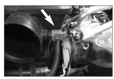
20a. Disconnect the air temperature electrical connection.
