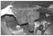
9. Lift the lower air box and remove it from the vehicle as shown.
