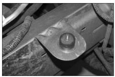
17. Using the two fender washers and one rubber washer, install the 6mm male/female rubber mounted stud onto the lower air box mount as shown.
