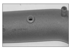
26. Install the supplied rubber grommet into the K&N intake tube as shown.
