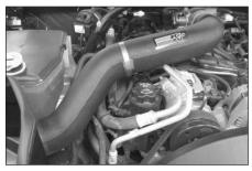
29. Install the K&N intake tube into the silicone hose at the throttle body and onto the saddle clamp, then secure with the provided hose clamps as shown.
