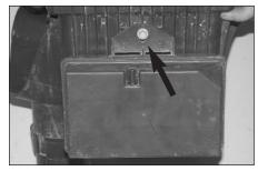
14. Remove the bolt which secures the vacuum reservoir to the air box and then remove the reservoir from the air box.
