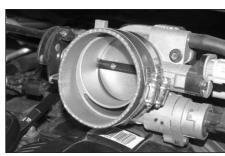
21. Install the silicone hose (08690) onto the throttle body and secure with the provided hose clamp.
