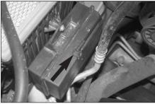
4. Disconnect the vacuum canister hose shown.
