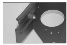
12. Install the bracket/rubber mounted stud assembly onto the heat shield as shown using the provided hardware.
