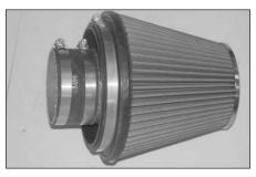
33. Install the silicone (08630) onto the air filter assembly and secure with the provided hose clamp.
