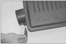
25. Rotate the air temperature sensor counter clockwise and remove the sensor from the stock intake plenum as shown.
