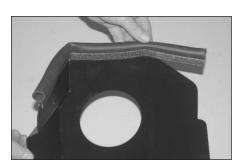
10. Install the provided edge trim onto the heat shield as shown. NOTE: Some trimming of the edge trim may be necessary.
