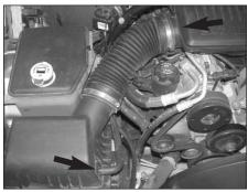
2. Loosen the hose clamp, which secures the stock intake tube to the intake plenum, and disconnect the crank case vent hose from the air box lid
