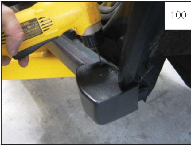
Drill marked holes with 3/32" drill bit.
