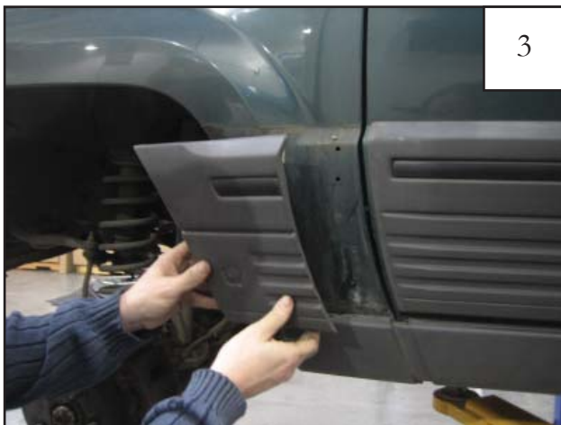
Remove upper factory side cladding piece from front fender.
