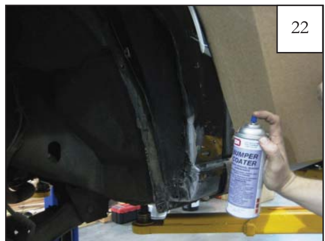
Using spray paint, repaint the sanded edge of the wheel well. NOTE: Be sure to cover the rest of the vehicle so paint does not get on other accessories such as side cladding.
