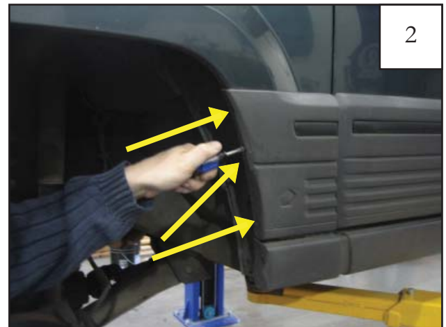
Remove factory screws from upper side cladding. Three places.
