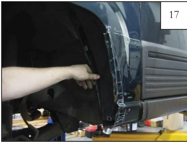
Push splash shield back into place.
