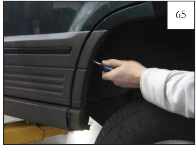
Remove small factory side cladding piece from "dog leg" area of rear wheel well.
