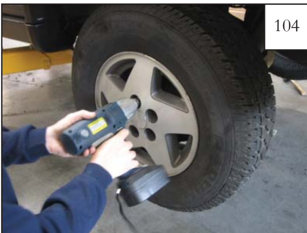
Reinstall the tire using an impact wrench.
