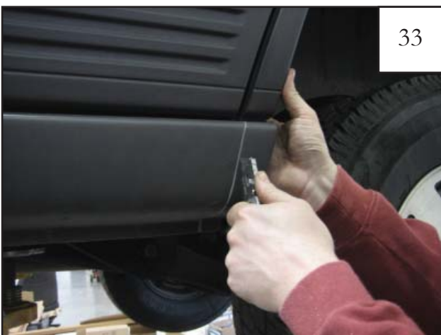
Mark a line parallel with the forward edge of the rear wheel well from the door seam down to pinch weld along the rocker panel. Using a utility knife, make several cuts to cut off end of rocker panel along marked line.
