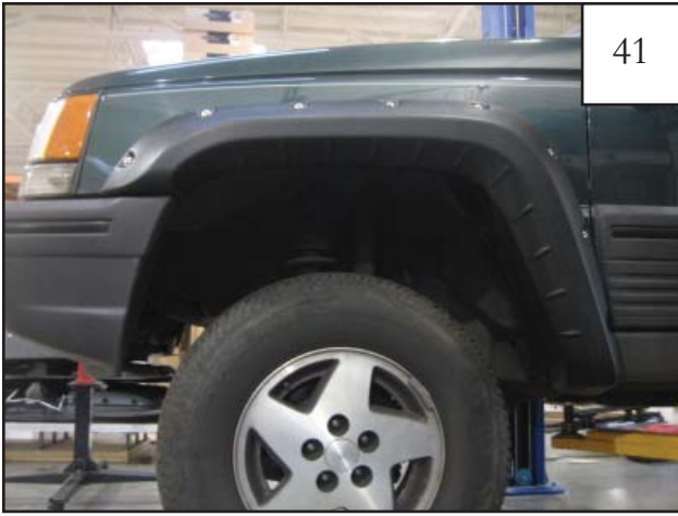
Completed front flare installation.
