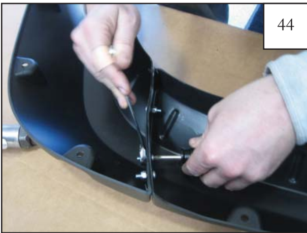
Once satisfied with alignment, tighten all screws.
