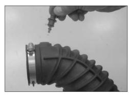
7. Remove the air temperature sensor from the stock intake tube as shown. NOTE: Take care when handling the air temperature sensor as it is very fragile.
