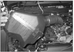
5. Lift up the air box assembly to dislodge it from the mounting grommets and then remove the complete assembly from the vehicle.
