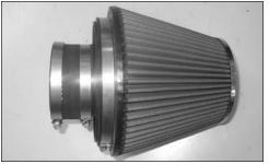
23. Install the silicone hose (08630) onto the air filter adapter and secure with the provided hose clamp.
