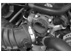
4. Loosen the hose clamp that secures the stock intake tube to the throttle body and then disconnect the intake tube from the throttle body.
