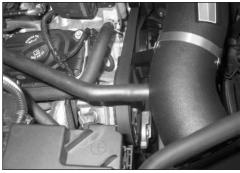
21. Connect the crank case vent hose to the K&N intake tube.
