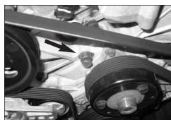
10. Remove the front engine bolt shown. NOTE: This bolt will be reused.
