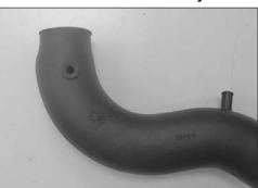
6. Install the supplied grommet into the hole in the K&N intake tube as shown.
