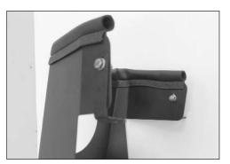
18. Install the supplied "L" bracket (07195) onto the heat shield as shown with the provided hardware.
