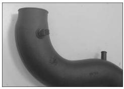
8. Install the air temperature sensor into the grommet installed into the K&N intake tube during step #6.
