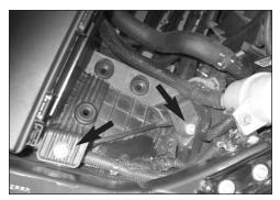
13.Remove the power steering reservoir mounting bolt and the two air box bracket mounting bolts shown.
