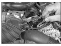
2. Release the locking tab on the air temperature sensor electrical connector and disconnect the connection.
