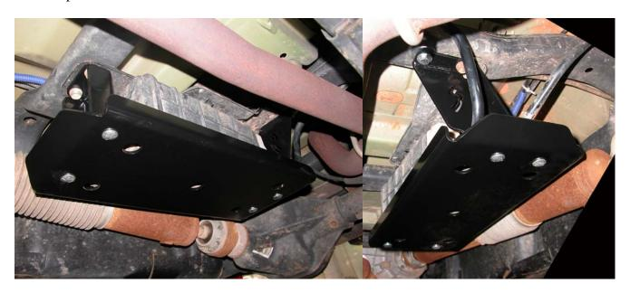
**Step 7:** Once all of the bolts are installed, tighten them. You may want to push the skid plate away from the driveshaft prior to tightening the bolts just to gain a little extra clearance.
