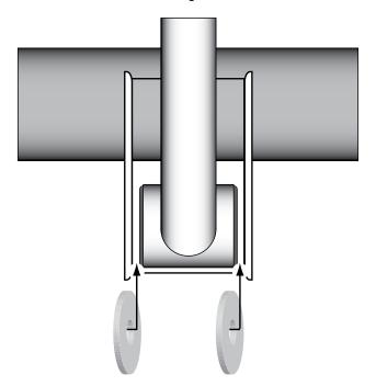
IMPORTANT: Each Control Arm requires (4) shim washers for installation. (2) 1/8" thick shim washers are required for the chassis end of the Control Arm, and (2) 1/4" thick shim washers are required for the axle end.
