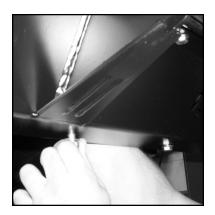
Start several of the bottom bolts into their holes with washers and nuts, and then remove the C-clamp or Vise-Grips that you had the plate clamped to the crossmember with.
