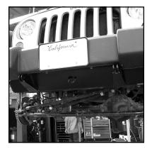
Before proceeding any further, center the new plate side to side on the vehicle using the bumper guards and the tow bar mounts on the plate as reference. Tighten the 4 top bolts.
