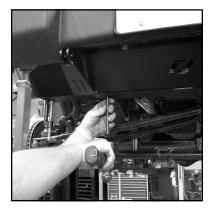
Using the plate as a template, and a 3/8" transfer punch, punch the 2 undrilled upper holes and all of the bottom holes.
