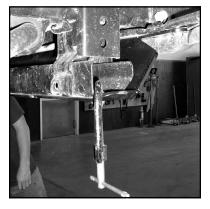
Next, with C-clamps or Vise-Grips, clamp the back of the plate up snuggly to the bottom of the crossmember.
