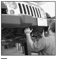
Fit new plate into position. Make sure the ends of the new plate wedge between the ends of the stock plastic bumper cover and the metal of the frame crossmember.
