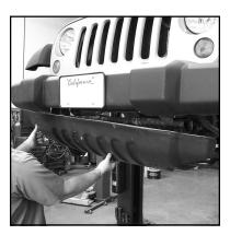
Remove all plastic attaching screws from stock plastic valance panel, then remove the panel from the vehicle.
