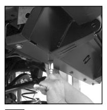
After all of the lower bolts are in their holes, go back and tighten all of the bolts with a 9/16" wrench on top and socket on the bottom.
