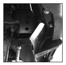
Install the remaining 2 top bolts, using the  $3/8''-24 \times 1''$  bolts, a washer top and bottom, and the nylock nuts. Go ahead and tighten these bolts down.
