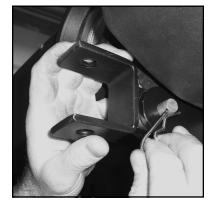
Attatch tow bar ends by inserting them into the bracket on the plate and affixing them in place with the clevis pins and hairpins. Tow bar ends must then be bolted to the tow bar of your choice.
