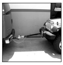
For optimum performance your tow vehicle's hitch should allow for the tow bar to ride as level as possible. Always use safety chains (included with the CE-9033F tow bar). This system will work with universal adjustable tow bars from Friedl, Draw-Tite, Valley, or Blue Ox.
