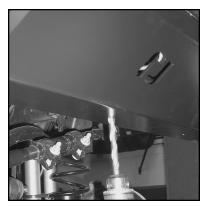
Now go back and drill the holes. Drill pilot holes first with a 3/16" bit, and then follow that up with a 3/8" bit.
