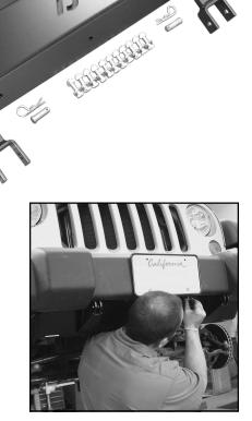
Initially mount the new plate to the bottom of the bumper by installing 4 of the 3/8"-24 x 1" bolts, washers top and bottom, and nylock nuts in the 4 pre-existing upper holes. Snug these bolts, but do not tighten.
