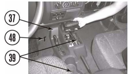
b. Install cup holder (38) on shift lever console (37).
