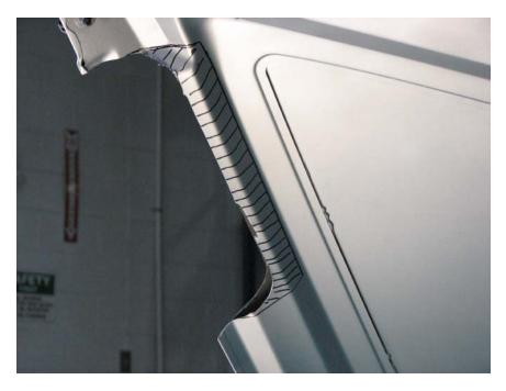
6. Using the cutoff wheel, clearance the hood inner so that it clears the opening when viewed from the side.
