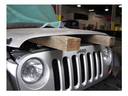
3. Use a pilot drill to drill both layers of the hood first, then use the 2" (50.8mm) hole saw to carefully cut through both layers of the hood.
