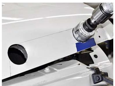
4. Using a cutoff wheel or reciprocating body saw, cut out the rest of the opening.
