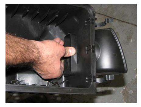
5. Cut off the small locator on the factory airbox (shown in gray below).
