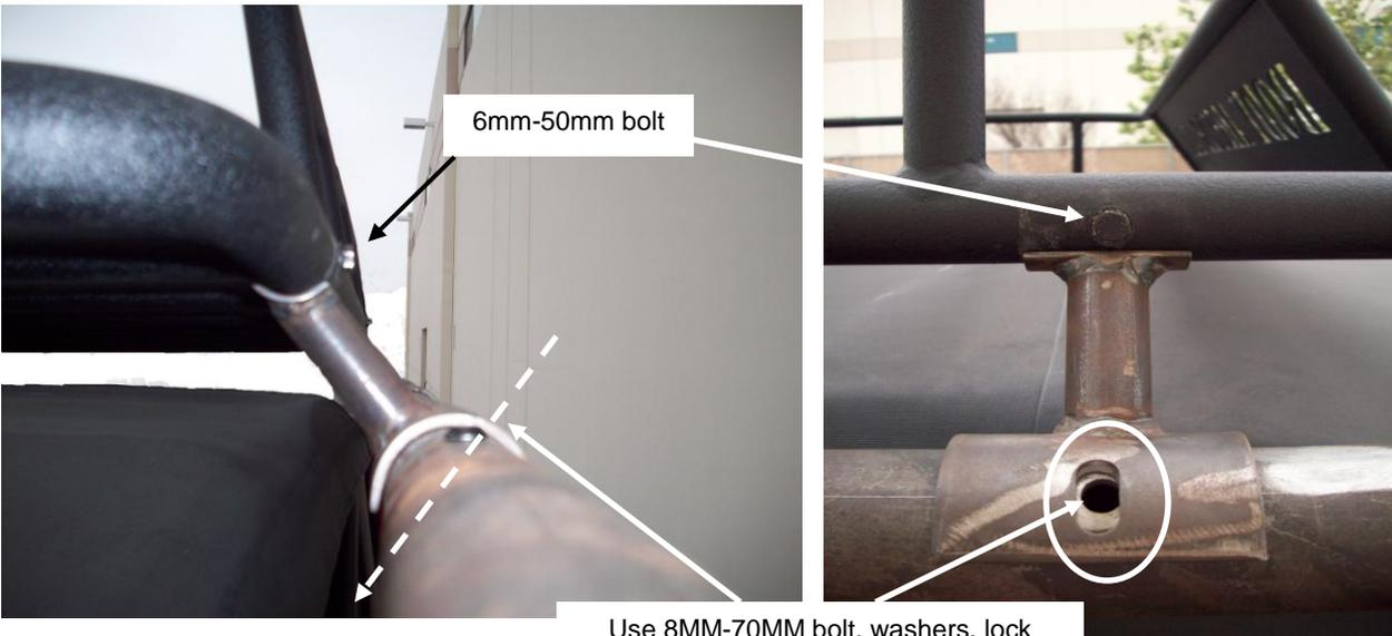
Use 8MM-70MM bolt, washers, lock washer and nut on each pedestal base
