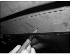
6. Re-install the rocker panel by using the 10mm button head bolts with flat washers, lock washers, and standard nuts for the side mounting holes. For the bottom three mounting holes, use the three hex head bolts with washers, spacers and nylock nuts. The long bolt goes in the bottom center hole with the 45mm spacer and the 2 medium bolts go in the front and rear bottom mounting holes with the 25mm spacer.
