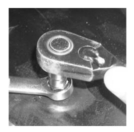
4. After drilling the side holes, Place the rocker panel against the side of the vehicle and use the 10mm black button head bolts with flat washers, and standard nuts on the inside of the vehicle. Do not use the lock washers yet as the rocker panel will be removed after marking the bottom holes. Hand tighten bolts evenly to secure the rocker panel in position.
