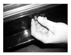
5. To mark the three bottom holes, stick a black marker through each hole and mark the vehicle making sure the mark is aligned vertically with the hole. Remove the rocker panels after the three bottom holes are marked. Use a center punch to mark each bottom hole so that from inside the vehicle, you can tell where the hole will be located. Before drilling, pull carpeting back and remove anything that might get in the way of the drill. Drill the three bottom holes to 7/16".
