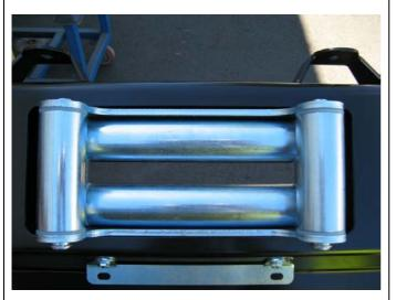
2. If fitting winch fit roller fair lead to front position in winch bumper
