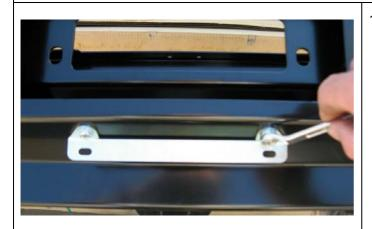
1. Fit licence plate bracket to mount face on lower front of winch bumper using holes provided.
