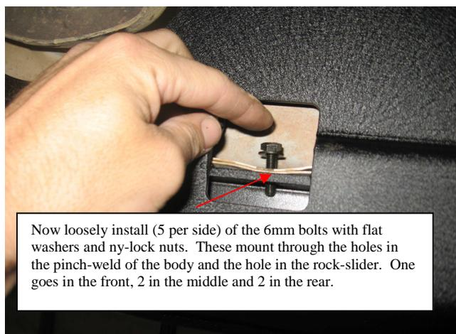
Now loosely install (5 per side) of the 6mm bolts with flat washers and ny-lock nuts. These mount through the holes in the pinch-weld of the body and the hole in the rock-slider. One goes in the front, 2 in the middle and 2 in the rear.
