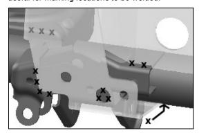
HINT: Be sure to include area on lower spring mount where it makes contact with Trackbar Brace. Also include back side of axle tube where Trackbar Brace wraps underneath.
