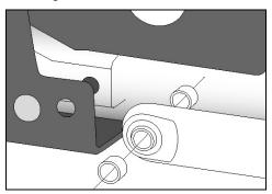
**HINT:** If necessary, install bushing/bearing spacers (not included) to ensure a proper fit between damper and mounting bracket.
