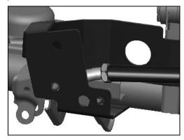
...or use the upper mounting hole if vehicle has a "drag link flip" or high-steering conversion. When track bar is installed in the upper hole, the supplied steel sleeve must be installed in the lower hole using the hardware provided.
