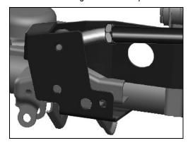
O Mount chassis end of track bar and loosely install the original mounting hardware.
