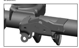
O Slide the Trackbar Brace over the factory track bar bracket as illustrated below. *HINT:* The Trackbar Brace is designed to provide a snug fit and may require some persuasion to maneuver into position.
