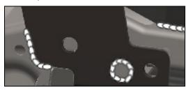
IMPORTANT: Avoid overheating axle tube and rubber bushing in vertical upper control arm mount by welding a small section and allowing the surface to cool off regularly.
