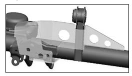
With the Trackbar Brace in position, insert one M12 x 70mm Bolt (C) into the original mounting hole as illustrated below. Secure the bolt with the original flag nut and temporarily tighten to hold the brace securely to the factory bracket.
