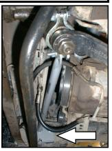
This steering brace fits 1987-2001 Jeep® XJ Cherokee vehicles with power steering, and 4.0L engines. It is designed to bolt into existing holes in the chassis, with minor drilling, and clamps to the steering box housing just above the sector shaft/pitman arm.
