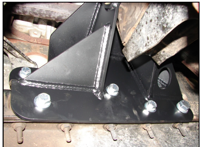
DS Block Bracket Installed
