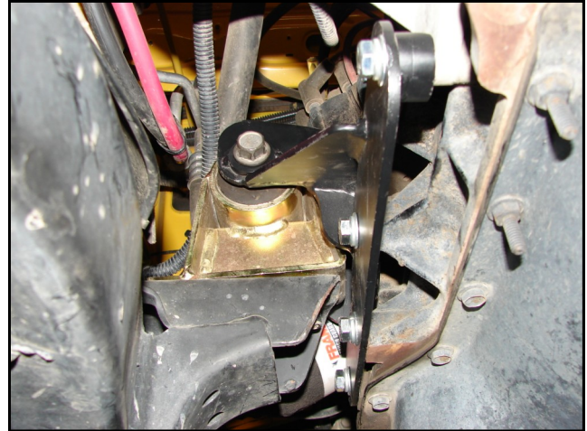
PS Block Bracket Installed
