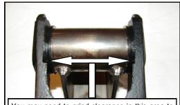
You may need to grind clearance in this area to allow the BombProof™ mount to fit into the factory "fork". More common on YJ's.
