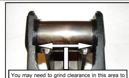
You may need to grind clearance in this area to allow the BombProof™ mount to fit into the factory "fork". More common on YJ's.
