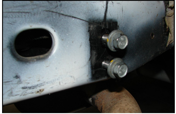
2– Factory bolts per side of frame.
