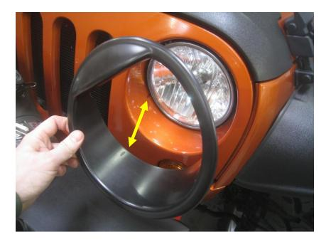
B) Hold the eyebrow bezel gently in place and peel the red backing away from the adhesive tape.
