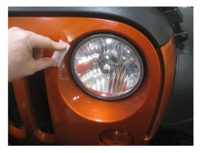
B) Fold the red vinyl backing from the adhesive tape over at a 45° angle.
