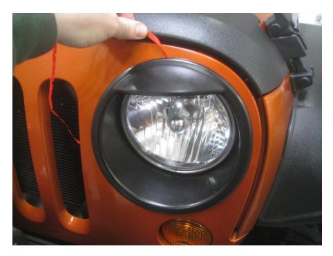
C) Apply firm pressure to the taped area all the way around the eyebrow bezel to ensure compressive contact of the adhesive to the grill.
