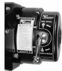
3-1: Clutch Engagement: SEC/PEC Models
