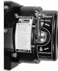
3-1: Clutch Engagement: SEC/PEC Models
