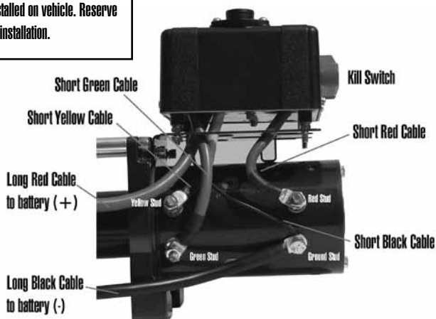
2-7: Complete Wiring Schematic: SEC8
