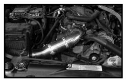
Step 14 Install the air intake tube by passing the filter end through the housing. Align the throttle body end of the tube with the coupler. Once the tube is aligned, fasten securely with supplied hose clamp. (Silicone based lubricants help locate the tube in the grommet.)
