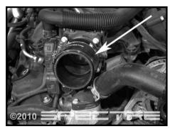
Step 10 Install the coupler over the coupler sleeve on throttle body and fasten securely with the supplied hose clamp. Install a second clamp but do not tighten at this time.
