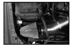
Step 16 Install the Spectre air filter and fasten securely with the supplied hose clamp. Ensure that all clamps and hardware are fully tightened at this time.
