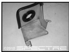
Step 12 Remove the three 10mm screws Dress the heatshield with the 3" grommet and the rubber seal.
