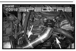
Step 15 Connect the crank case vent hose to the intake tube fitting. Reconnect the wiring harness for the air temperature sensor.
