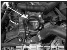
Step 9 Install the coupler sleeve onto the throttle body.
