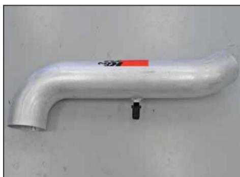
19. Install the provided NPT vent fitting into the K&N® intake tube as shown.
