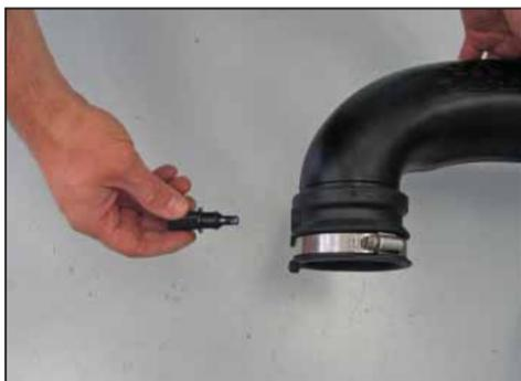
21. Remove inlet air temperature sensor from factory tube as shown.
