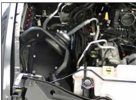
18. Place the heat shield assembly into vehicle so the mounting standoffs are secured in the factory airbox mounting grommets. Secure the mounting bracket to the ECU using the bolt removed in step #17.
