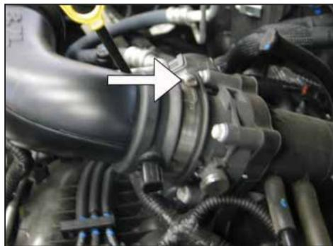
5. Loosen hose clamp at throttle body.
