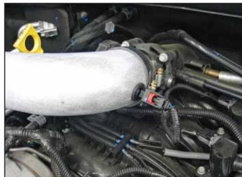
27. Reconnect the inlet air temperature sensor electrical connector as shown.
