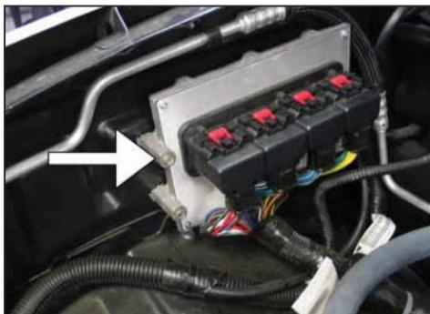
17. Remove the front upper ECU mounting bolt shown.
