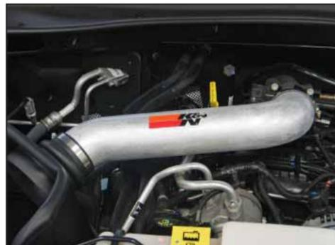
23. Install K&N® intake tube into the silicone hose at the filter adapter and then into the silicone hose on the throttle body. Secure the intake tube with the provided hose clamps.
