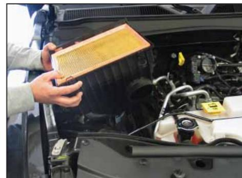
7. Lift up the lower airbox assembly to dislodge it from the mounting grommets, then disconnect the fresh air duct from the lower airbox and then remove the lower airbox from the vehicle.
