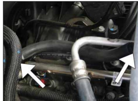
25. Install the crankcase vent hose onto the NPT fitting on the K&N® intake tube. Install the hose mender end into the factory elbow on the valve cover.
