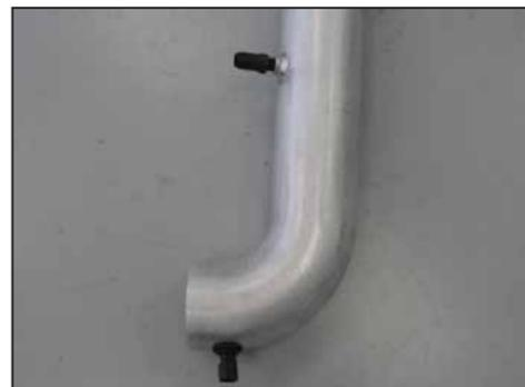
22. Install the inlet air temperature sensor into the grommet previously installed during step #21.
