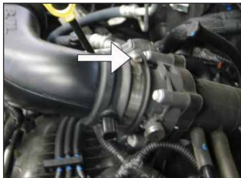
5. Loosen hose clamp at throttle body.
