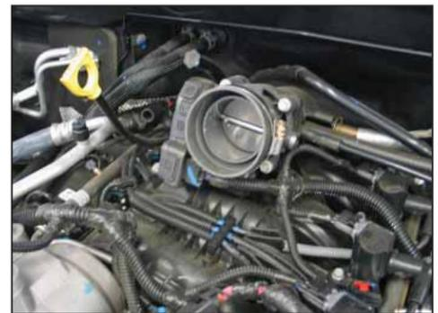
8. Install hose the silicone hose (084034) onto the throttle body and secure with the provided hose clamp.
