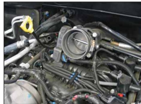
8. Install hose the silicone hose (084034) onto the throttle body and secure with the provided hose clamp.
