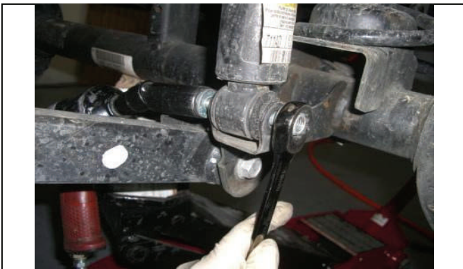
Disconnect and remove front lower shock hardware.
