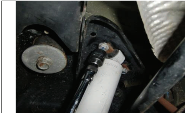
Next, remove rear upper shock bolts.
