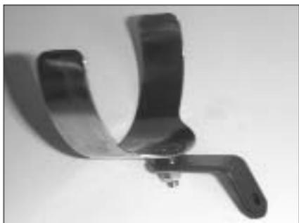
14. Assemble the saddle and "L" bracket using the hardware provided.
