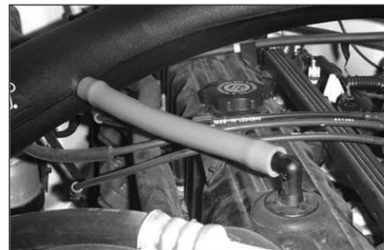
23. Attach the vent hose provided onto the vent fitting on the valve cover and the K&N intake tube.
