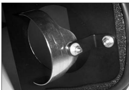
15. Attach the saddle bracket assembly to the heat shield using the hardware provided. **Note: Do not tighten completely at this time.**
