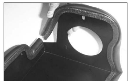
9. Install trim seal onto the heat shield. **Note: Some cutting and trimming will be necessary to achieve best fit.**
