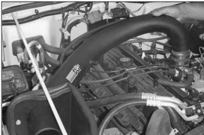
19. Install the K&N intake tube.
