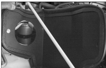
16. Install the heat shield assembly.
