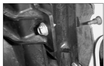
11. Loosen and remove the upper radiator shroud retaining bolt.
