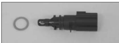
5a. Remove the sealing o-ring from the temperature sensor as shown.
