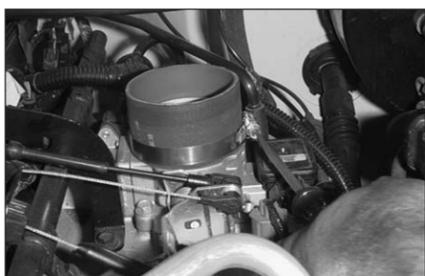
18. Attach the silicone hose to the throttle body using a hose clamp provided.
