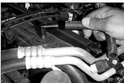
22. Detach the crankcase vent hose from the vent fitting on the valve cover.
