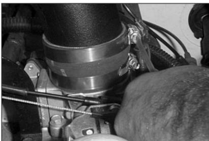
21. Tighten the hose clamp on the silicone hose at the intake tube.
