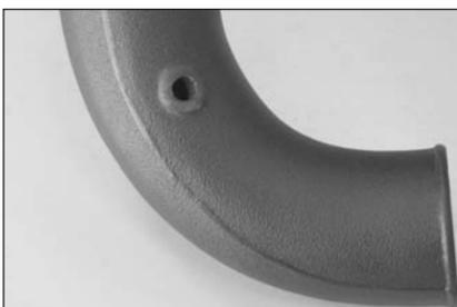
19b. Remove the K&N intake tube from the vehicle and drill a 3/4" hole at the position marked in step #19a. Next install the provided grommet into the drilled hole.
