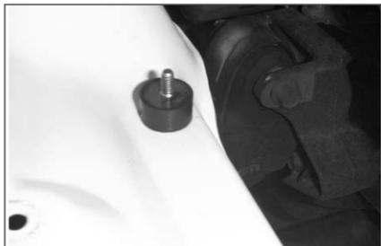
13. Install the second rubber mounted stud into the lower airbox mounting point using the hardware provided.
