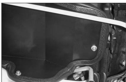
17. Secure the heat shield to the rubber mounted studs using the hardware provided.
