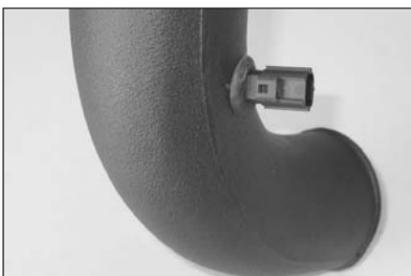
19c. Install the temperature sensor into the grommet as shown. **NOTE: The temperature sensor is fragile, handle with care.**
