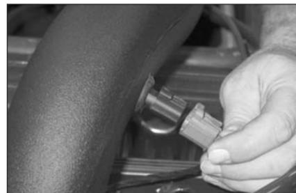
23a. Reconnect the temperature sensor electrical connection.
