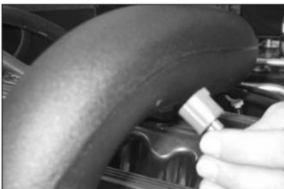
19a. Position the temperature sensor electrical connector next to the K&N intake tube for the best fit, then mark the location for drilled.
