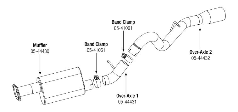
**Step 1: (Read Instructions prior to installation)** Remove your stock exhaust from the rear of your truck working your way forward. Take caution not to damage the factory isolation mounts as they will be reused. It may be helpful to lubricate the isolation mounts prior to disassembly. It is recommended to not fully tighten the clamps until the entire system has been installed.
