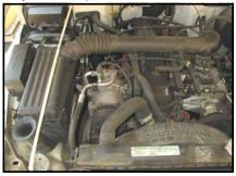
2. Remove the 1/2" crankcase vent hose from the OE air tube.
