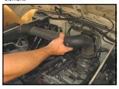
6. Loosen the 3 nuts that secure the OE air box to the inner fender of the vehicle.
