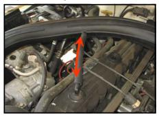
**If Equipped:** Remove the o-ring from the Air Temp. sensor before inserting the sensor into the grommet in the in-
