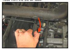
2a. **If Equipped:** Disconnect the Air Temp. Sensor electrical connection near the throttle body and rotate it a 1/4 turn counterclockwise to remove it from the tube..
