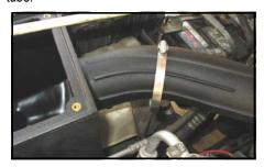
12. Install the S&B filter into the S&B box. Slide the filter onto the air tube until the filter base contacts the air box wall. This is a "pull thru method".
