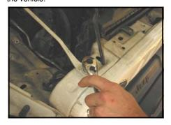
9. Install the S&B air box. Use the 1/4 bolts, washers, nuts and tighten the box to the inner fender.
