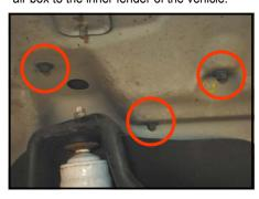
7. Remove the OE air box from the vehicle.
