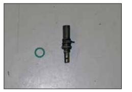
18. Remove the factory O-ring from the inlet air temperature sensor and replace with the O-ring provided.
