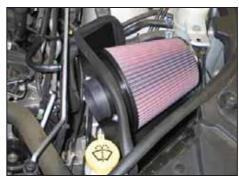
16. Set the heat shield/filter assembly into position so that the mounting grommets slide over the outer airbox mounting studs.
