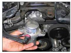
9. Remove the two nuts that secure the air injection pump to the mounting bracket. Gently set the air injection pump aside.
