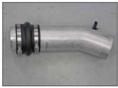
23. Slide the provided silicone hump hose (5-576) all the way onto the K&N $^{\odot}$  intake tube #27446 as shown.
