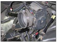
22. Install the provided silicone hose (08690) onto the throttle body and secure with the provided hose clamp.
