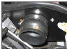
21. Install the provided hump hose (084057) onto to the filter adapter and secure with provided hose clamp.
