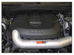
28. Adjust the intake kit for proper fit and then secure the mounting hardware and hose clamps. Reinstall the factory engine cover.
