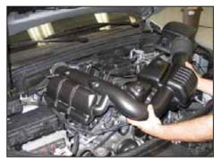
6. Remove the intake tube and upper airbox from the vehicle as shown.
