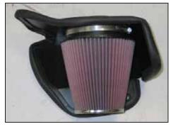
15. Install the K&N<sup>®</sup> air filter onto the filter adapter and secure with the provided hose clamp.
