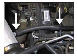
27. Install the provided crankcase vent hose onto the vent fitting installed into the K&N<sup>®</sup> intake tube, then connect the open end onto the crankcase vent tube cut in the previous step.
