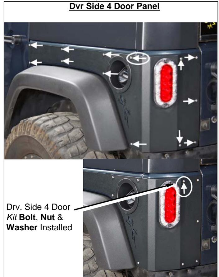
**\*\*Align and tighten all the *kit button head bolts*\*\***
