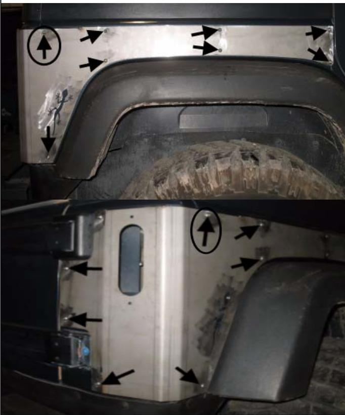
**h.** Mark both lower LED mounting holes for drilling out to 9/16" once you have removed *kit armor* panels.
