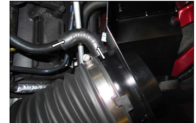
15. On V6 motors, connect the factory crankcase breather hard line to the Airaid Intake Tube using the 90 deg. Breather Elbow (#7). Disregard the 13" Breather Hose (#6) it will not be used.
