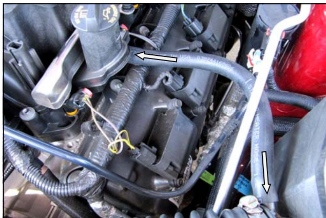
14. On V8 motors, replace the factory crankcase breather line with the 13" Breather Hose (#5) and connect it to the Airaid Intake Tube. Disregard the 90 deg. Elbow (#7) it will not be used.
