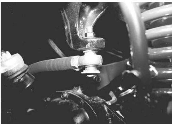
**Heavy Duty Tie Rod Tube Part # TR300**
