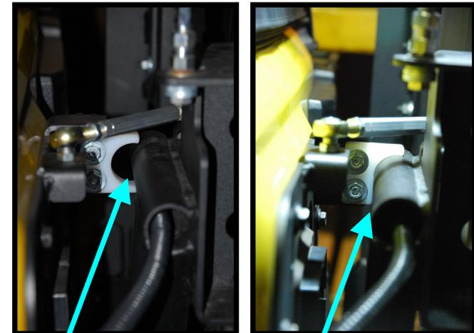
Step 10 – Tighten 5/16” bolts in Alignment Block & tighten 3/8” thin hex nuts against the connector rod. This will keep the connector rod from unthreading. You can also tighten the four Tailgate Bracket bolts.
