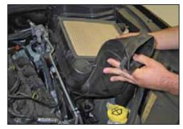
9. Lift up the lower airbox to dislodge it from the mounting grommets and then remove the lower airbox from the vehicle.
