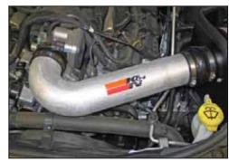
21. Install the K&N<sup>®</sup> intake tube into the silicone hump hose and then into the silicone hose at the throttle body, secure the intake tube with the provided hose clamp.
