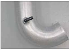
20. Install the 90° npt fitting into the  $K\&N^{\ensuremath{\mathbb{S}}}$  intake tube as shown.
