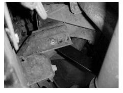
**Step 6:** Take the strut rod and attach it between the motor mount and the skid plate. Use one 3/8-16 bolt, lock washer, and nut to bolt it to the front of the skid plate and use the remaining ½-13 bolt, washer and nut to attach it to the rear of the motor mount. The view in the photo to the left is from the rear on the driver's side.
