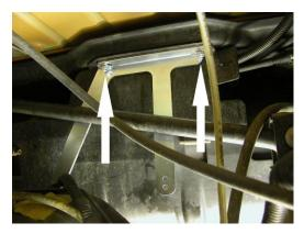
**Step 4:** Raise the skid plate into position under the gas tank using a floor jack. While raising the skid plate fit the two carriage bolts at the front of the skid plate into the holes in the front bracket. Use the lowermost holes on the bracket. Push the skid plate as far rearward as possible for maximum differential clearance. Also, push the skid plate as far as possible to the driver's side to gain clearance for the exhaust system. However, it probably won't move much.
