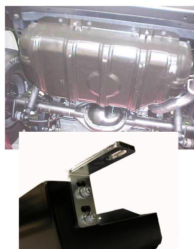
**Step 2:** Insert the remaining two 5/16-18x1.0" carriage bolts into the two square holes at the front of the skid plate with the threads facing outward. Place a small piece of tape around the threads to prevent them from falling out while positioning the skid plate as shown to the right.
