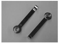
**Step 1:** Loosely attach both rear mounting brackets to the skid plate using the 5/16-18x1.0" carriage bolts, 5/16-18 nuts, and washers provided. The bolts should be installed from the inside of the skid plate. The longer bracket is installed on the passenger side of the vehicle to reach over the exhaust pipe. In addition, use the lowest slots in the brackets so that the top of the brackets are above the top of the skid plate side as shown in the photos below.
