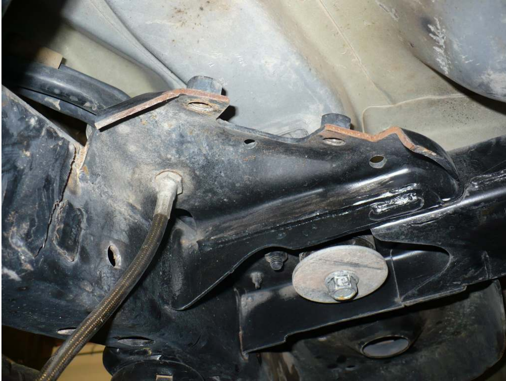
Picture 2.2 Example of properly trimmed stock shock mount
