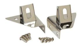
Remove the four bolts on the upper portion of the windshield hinge. Place the light bracket over the upper hinge and align the holes. Using the Stainless bolts provided start all four bolts then tighten evenly. We recommend that you use anti-sieze on all threads of the stainless bolts provided with your parts.
