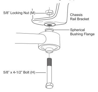
O Tighten the 5/8" x 4-1/2" Bolt (H) to 135 ft-lb. using a torque wrench.
