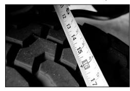
**HINT**: For example, measure from the edge of a tire tread lug to the outboard side of the chassis, then repeat the measurement on the other side of vehicle using the <u>exact</u> same points.
